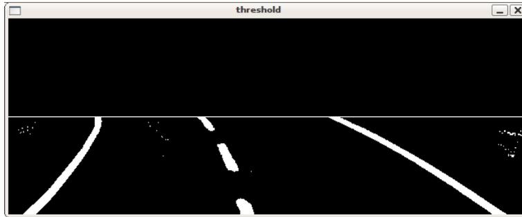
Figure 3.5: Binary road image after an adaptive threshold operation with virtual horizon
